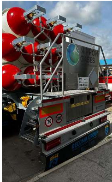
Hydrogen high flowrate tube trailer
