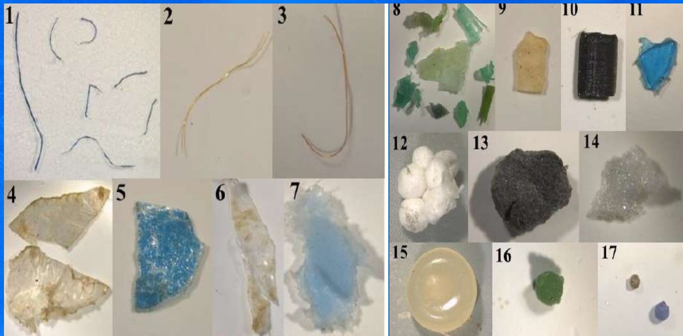
Figure 4: Common shapes of microplastics. (1: fibers, 2-3: filaments, 4-7: films, 8-11: fragments, 12-14: foams, 15: pellet, 16-17: granule) (Photo: © Ülgen Aytan, Turkey).
